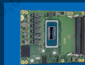
BGA/chip-down COM-HPC design example
