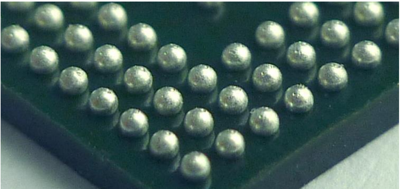
Figure 10: BGA package (bottom side)
