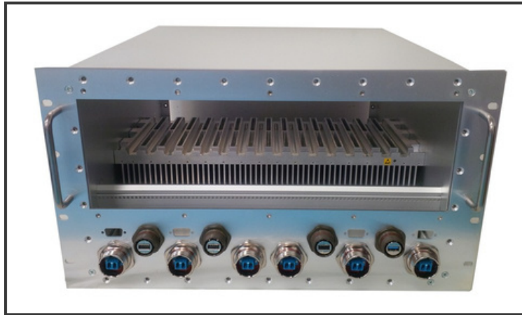
Figure 4: A card mat that employs “fins” to dissipate heat can be employed in a chassis, keeping the airflow on the outside of the card cage, but providing a way to cool the hotter modules in a system.
