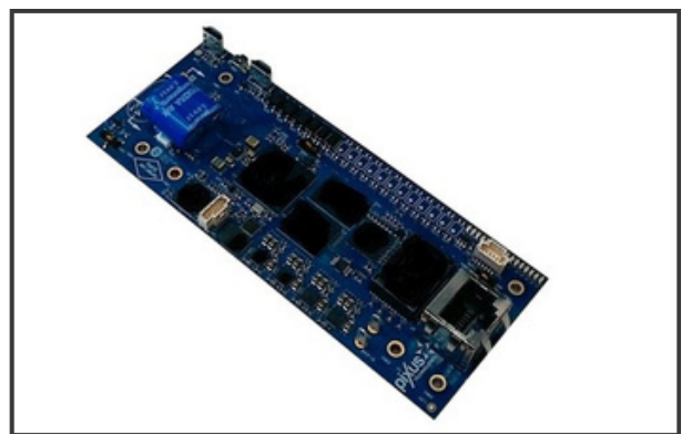
Figure 3b: A mezzanine-based approach can reside beneath the backplane and be mounted to it, this saves slot space inside the enclosure
