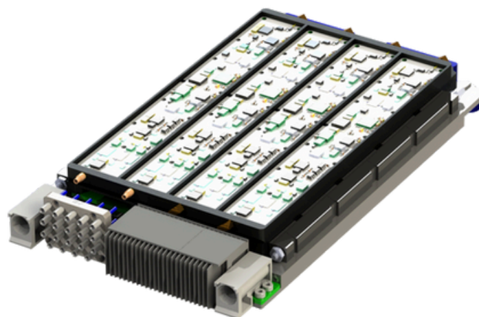
Figure 2: A SOSA-aligned 3U VPX module with flexible RF-on mezzanine architecture meets the SWaP-C requirements of modern military and aerospace systems
