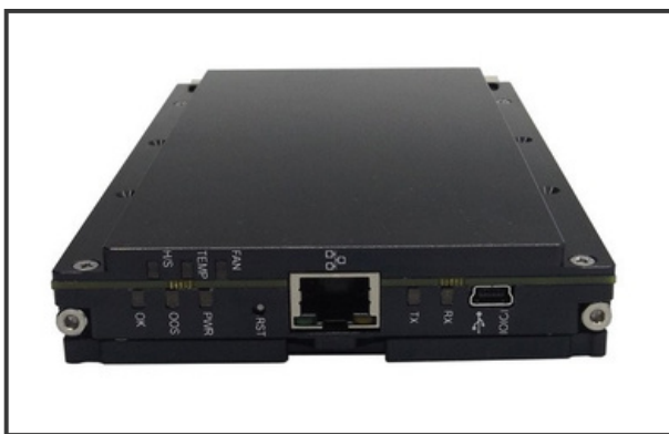
Figure 3a: Chassis management is a requirement for most SOSA aligned enclosure systems. A chassis manager can come in a pluggable form, but this consumes a slot
