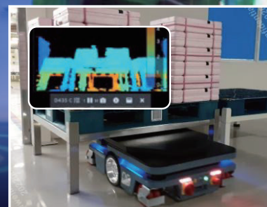
Real-Time AI Vision Analysis : pallet pick up
