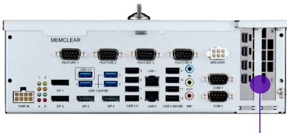
Dual-slot PEG Card Support (*Intel® Core™ Ultra 5 336H 4Xe SKU)
