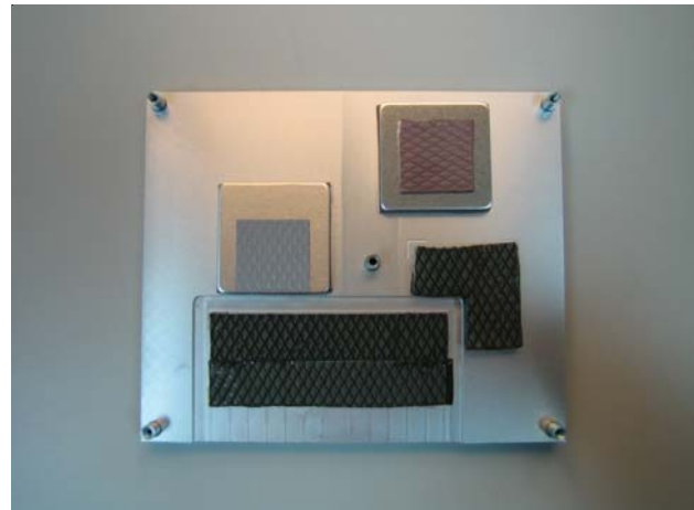
Pads for CPU, Northbridge, and Southbridge
