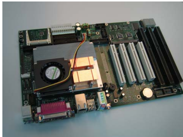
THSF-NR667-B installed on ETX-NR667 and ETX-carrier board.
