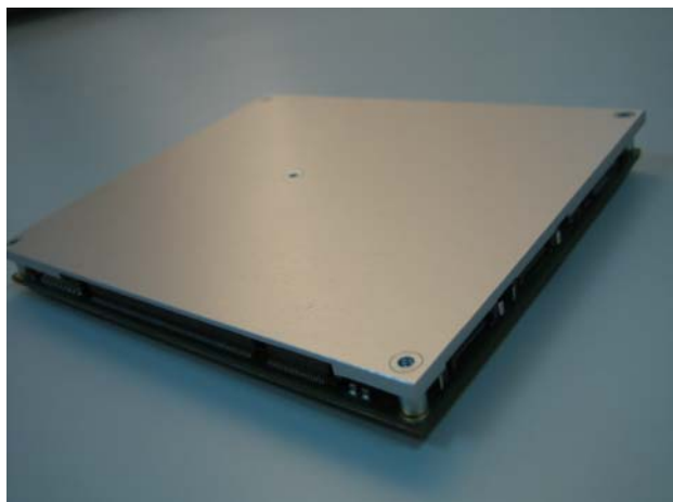
Heatspreader placed on ETX-NR667.
