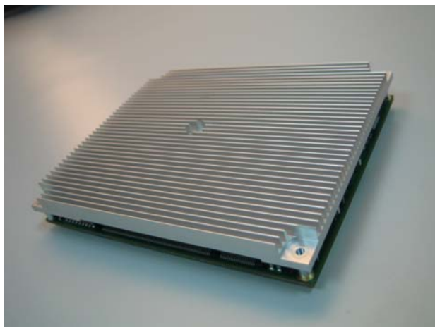
Heatsink mounted on ETX-NR667
