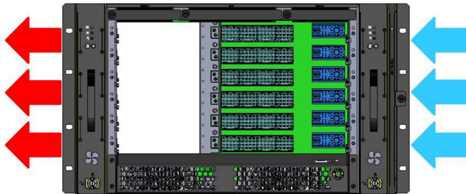
Figure 9: General airflow path for the 6U 6 slot ATCA Shelf
