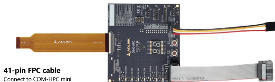
Figure 3 – Debug board and cable connections
