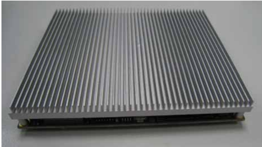
THS-EAT-B Low Profile Heatsink mounted on ETX-AT
