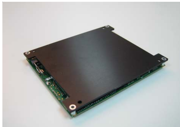
Heatspreader placed on ETX-GLX.
