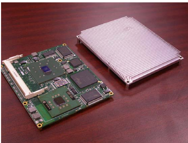
THSF-IM333-T heatsink with ETX-IM333-P1400
