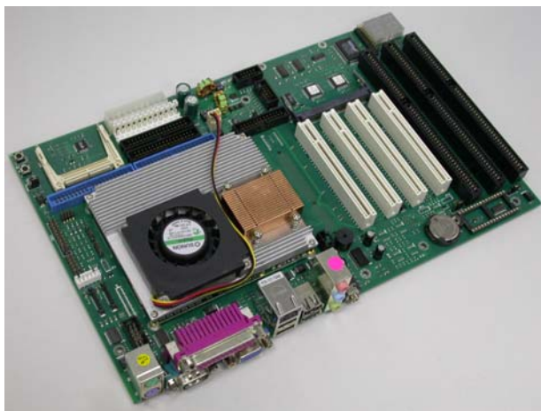
THSF-IM333 installed on ETX-IM333 and ETX-carrier board.
