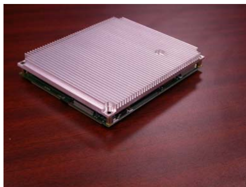
Heatsink mounted on ETX-IM333
