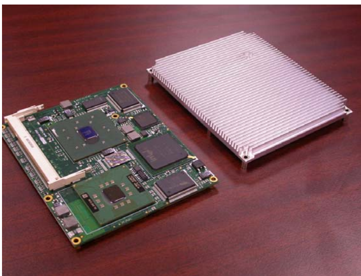
THSF-IM333-T heatsink with ETX-IM333-P1400
