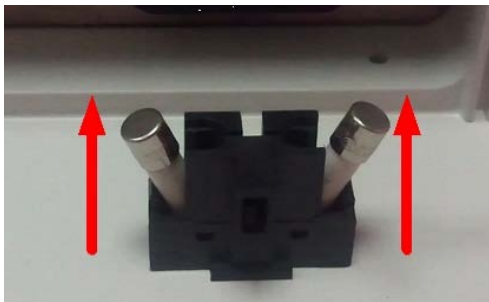
Figure 2-3: Removing unlocked fuses
