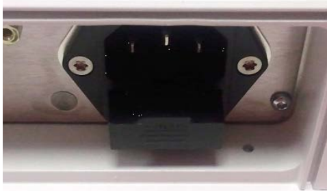
Figure 2-6: Re-inserting the fuse bracket
