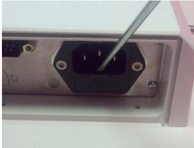
Figure 2-1: Removing fuse bracket
