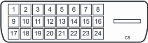
Figure 1-12: DVI-D Connector Pin Assignment
