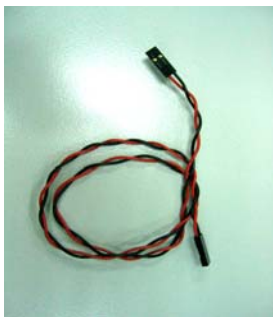
Figure 2-2: Watchdog reset cable
