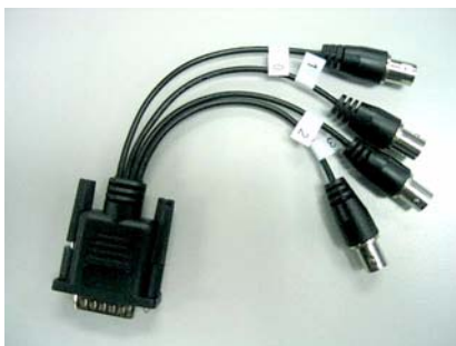
Figure 2-3: BNG Interface cable
