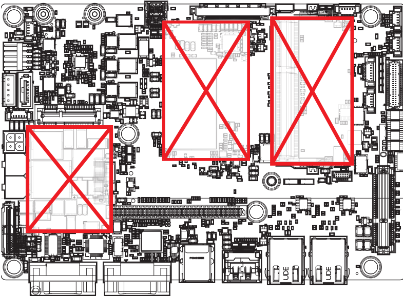
Figure 2-7: Cable Routing Considerations for Heat Sinks
