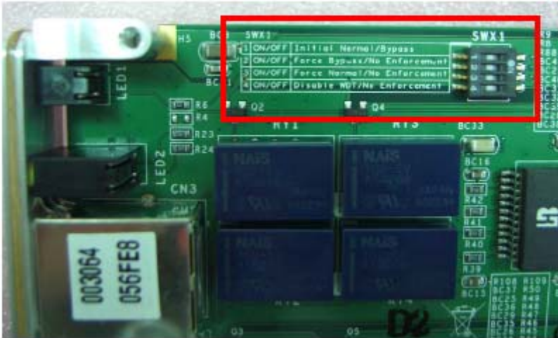
Figure 2-2: Control Switch (SWX1) & Pin Descriptions
