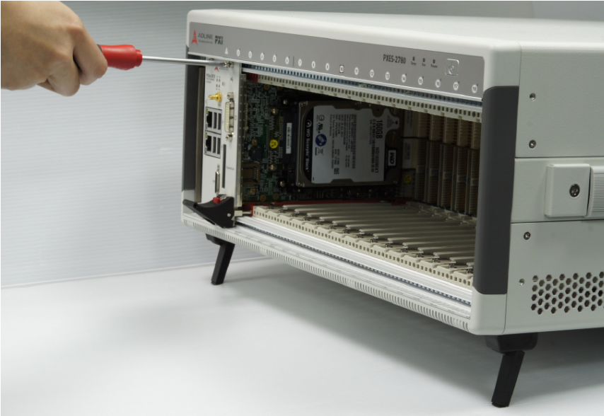
Figure 2-5: Fasten System Controller Module Screws
