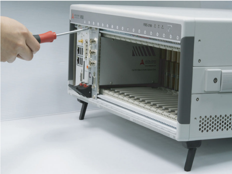
Figure 2-8: Fasten Peripheral Controller Module Screws
