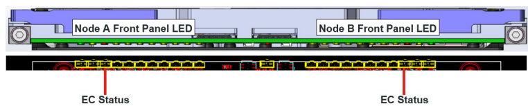
Figure 3-8: VPX6200 EC Status LED
