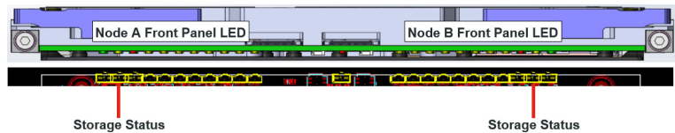
Figure 3-7: VPX6200 Storage Status LED
