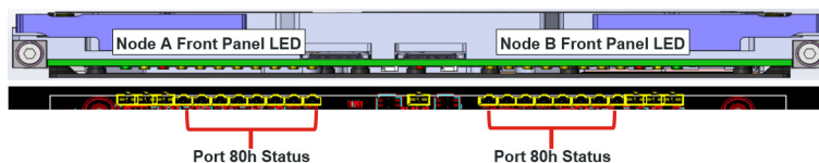
Figure 3-9: VPX6200 Port 80h Status LED
